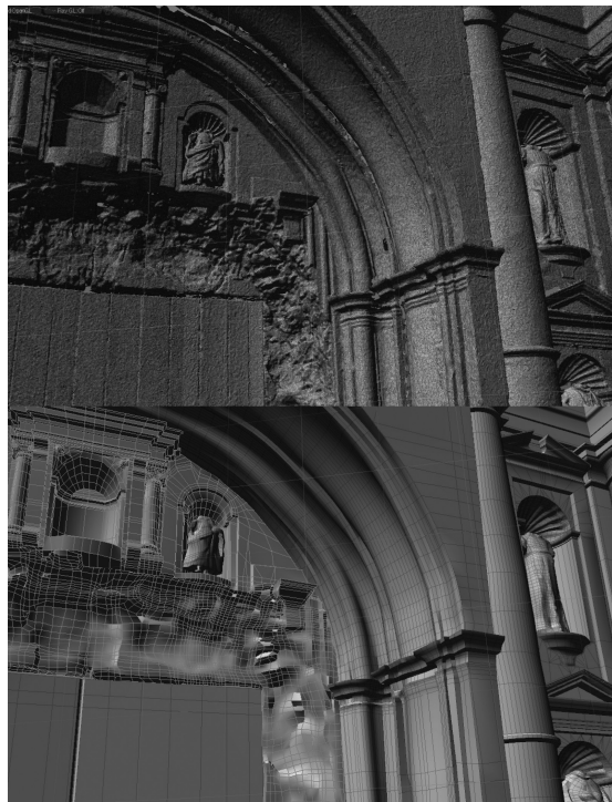
Fig. 1. II The process of data decimation ( iglesia de la Compañia de Jesus , Antigua Guatemala). 3D models are ' simulacra ' of reality and as such a version that always gives back partial information; this statement is also valid for morphometric data. According to the purpose for which a 3D model is realised, the amount of initial data is decimated, both because it is in fact unmanageable with today's hardware , and second because it is generally not necessary to describe with such attention an architectural artefact (depending on the exported scale—see Senatore 2011, pp. 47). The more the operator acts on the initial data, the more the final 3D model will shift from the real object's geometry; the data related to the morphometric deviation between the 3D 'point cloud' model (the raw starting data) and the models that can be deduced from this, make it possible to verify the reliability of the latter
