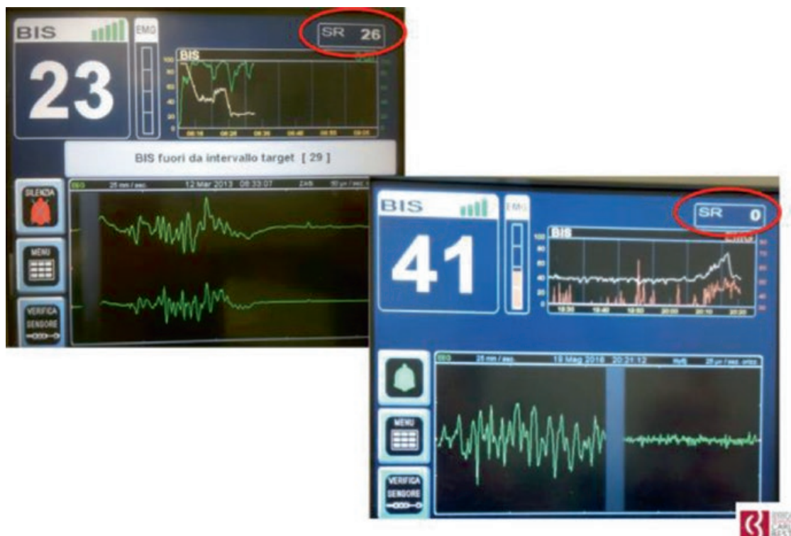
Fig. 5.10 Burst suppression rhythm without artifacts (left) and with artifacts (right) created by a coagulator. The small and rapid frequency waves on the flat portion of EEG falsely increase the qEEG number. Their presence is signaled by the red signal increasing on the EMG bar and is recognizable on the trend. The red circle highlights the SR
