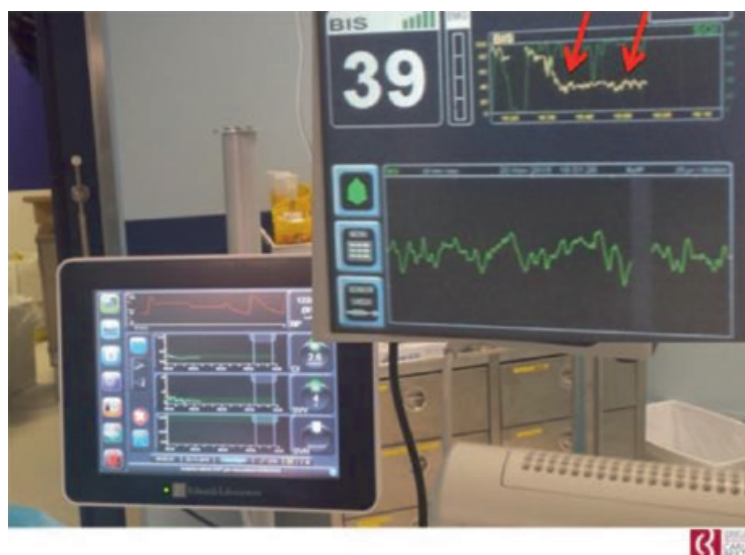
Fig. 5.16 Trend BIS (i.e., the numerical sequence in the time of qEEG values) remains stable (red arrows) after painful stimulation (intubation and vascular accesses)
