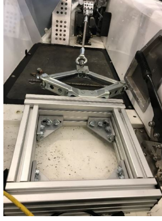
(b) Frame attached to the seat mounting points
