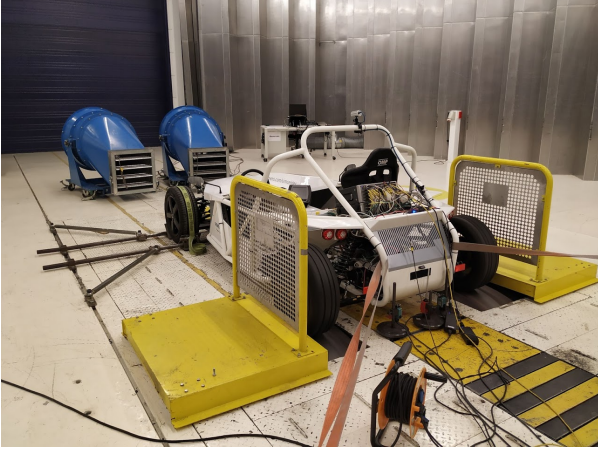
(a) SimRod installed on the chassis dynamometer during the rear-left brake testing
