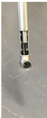
Figure 69, a picture of the Kiel probe equipped with a thermocouple used in the rig, suitable for high temperature applications
