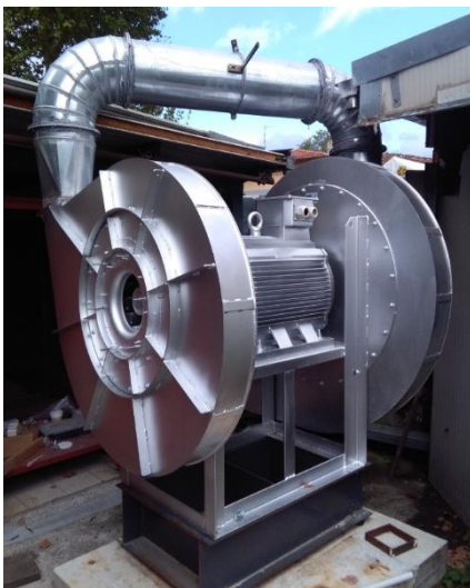
Figure 21 Fan, installed at UniFi grazing flow test rig laboratory
