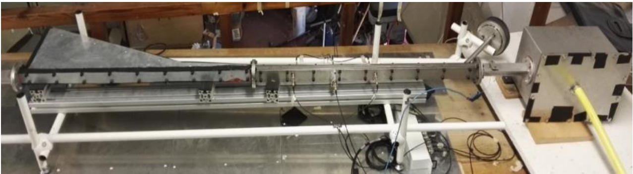
Figure 82, calibration test rig for acoustic measurements
