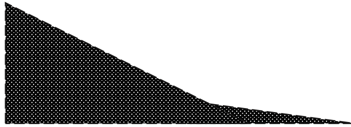
Figure 37, typical shape of a 2-slope anechoic termination
