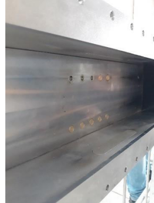
Figure 81, microphones installed on the rig, duct inner view
