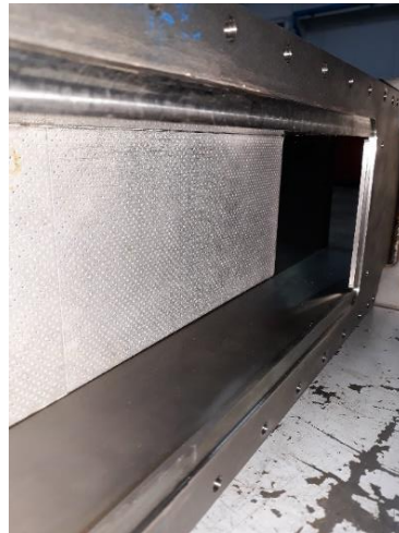
Figure 59, acoustic liner installation on the dedicated window in the test section
