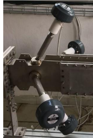
Figure 62, speakers installed on the rig
