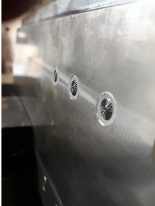
Figure 80, flush mounted microphones on the duct wall
