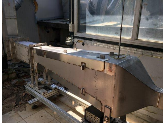
Figure 36, plenum installed on the test rig
