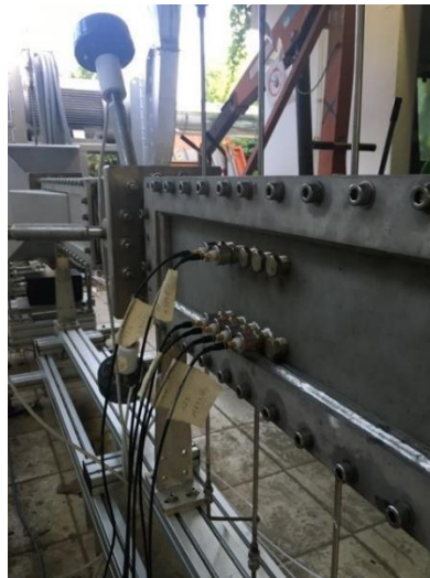
Figure 79, a picture of microphones and taps installed on the rig
