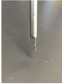
Figure 72, a picture of 2-dimensional 3-hole probe
