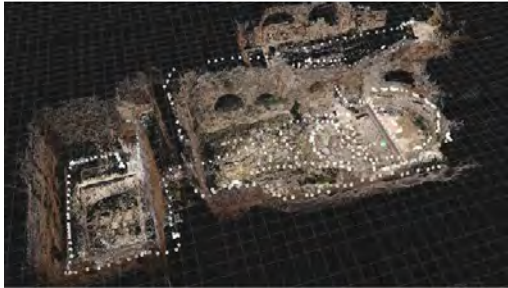
Fig. 11 – Salmis central calidarium, Terrestrial Digital Photogrammetric survey section (Copyright: Camiz, Tedeschi, Griffo 2018).
