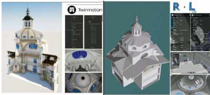
Fig. 14 Comparison between the two plugins (twinmotion and revit live) for the interactive visualization of the H-BIM model
