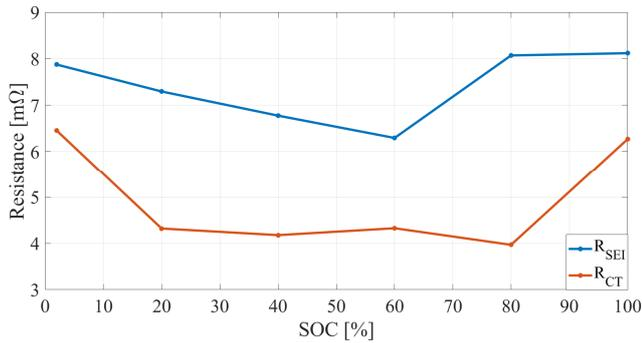
Fig. 4. Dependence of battery SEI resistance and charge-transfer resistance ( $R_{SEI}, R_{CT}$ ) at different SOC (cell #5, SOH=60%).
