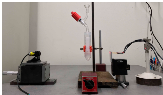
Figure 1. Setup for light transmittance measurements. By moving the vial up or down, the laser is allowed to go through the upper or the lower phase.
