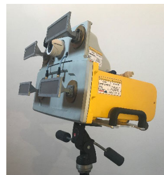
FIGURE 4. Radar configuration with four antennas connected.
