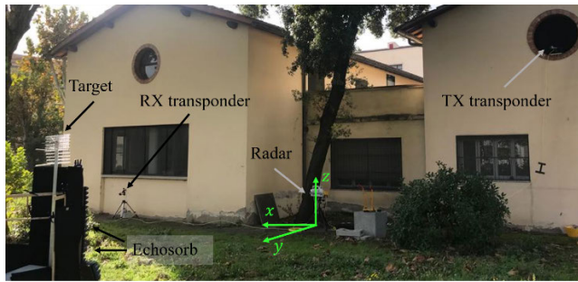
FIGURE 6. Radar installation in controlled scenario.
