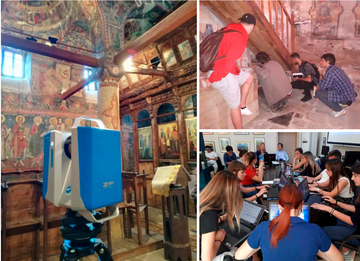
Figure 0-4 Left: The laser scanner running in the interior of the Church of Dormition of Mary in Leusë. Right, above: During the survey. Right, below: Digital survey data processing at the Multifunctional Centre in Përmet.
