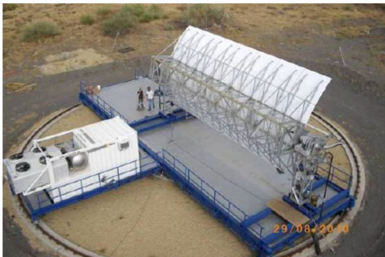
Figure 1.16: Kontas rotating platform at PSA [43].
