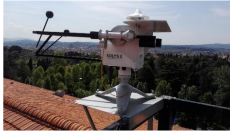
Figure 4.7: The two axes sun tracker with one pyrheliometer and two pyranometer.
