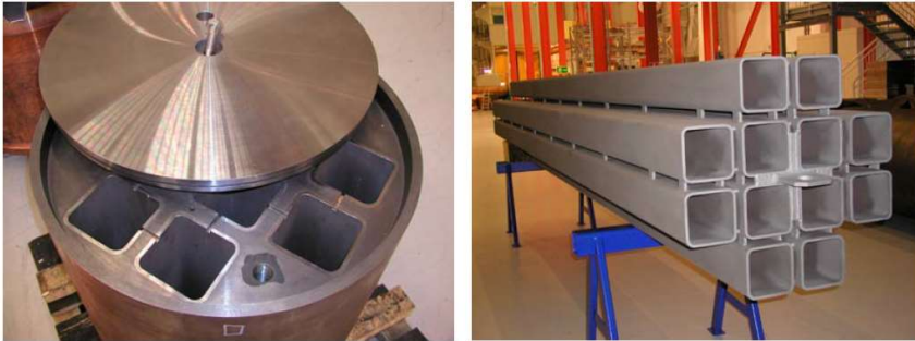
Figure 16 Part of the machined insert with the notches between the fuel channels and a steel lid (on the left) and a steel tube cassette for hosting fuel assemblies (on the right).
