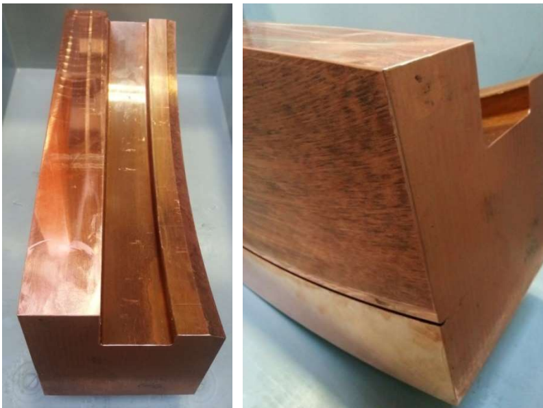
Figure 47 Views of the copper flange investigated by ultrasound.
