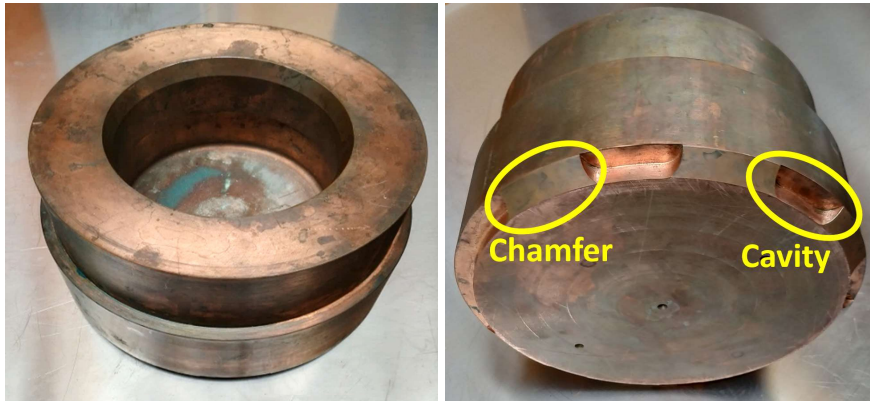
Figure 30 Mock-up of the copper lid with a \frac{1}{4} scaled diameter but the same thickness of a full-scale lid (on the left). View of the bottom surface of the mock-up where chamfers and cavities are realized.
