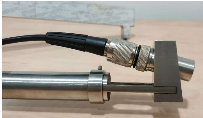
Figure 87 Probe holder with a 15^\circ inclined hole to host the transducer and a 7.5^\circ inclined surface, to split the ultrasonic beam into two directions.
