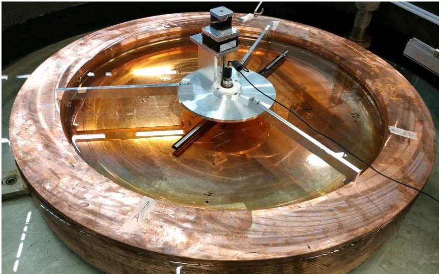
Figure 66 Ultrasonic acquisition device placed above a copper sample for inspections.
