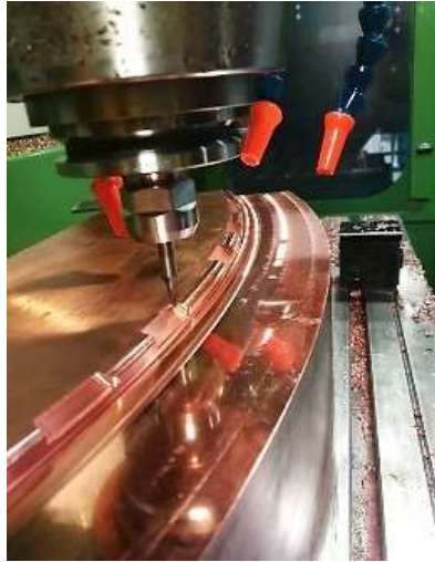
Figure 90 Manufacturing of chamfers on a copper flange by a CNC machine.
