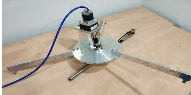
Figure 86 Ultrasonic reader prototype for the recording of both the identification and the authentication fingerprints.
