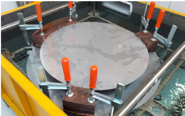
Figure 50 Copper flanges arranged around a circumference in order to reproduce the full copper lid geometry.
