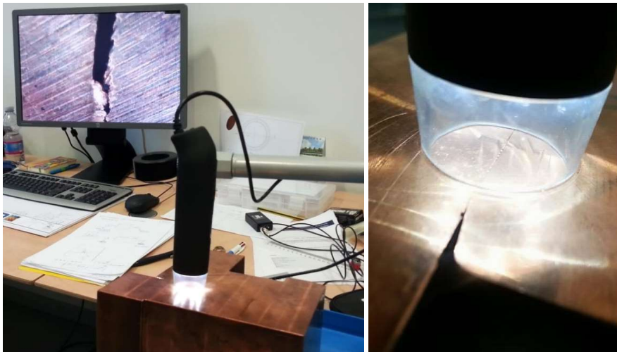
Figure 21 Set-up of measurements for optical inspection by a digital microscope.
