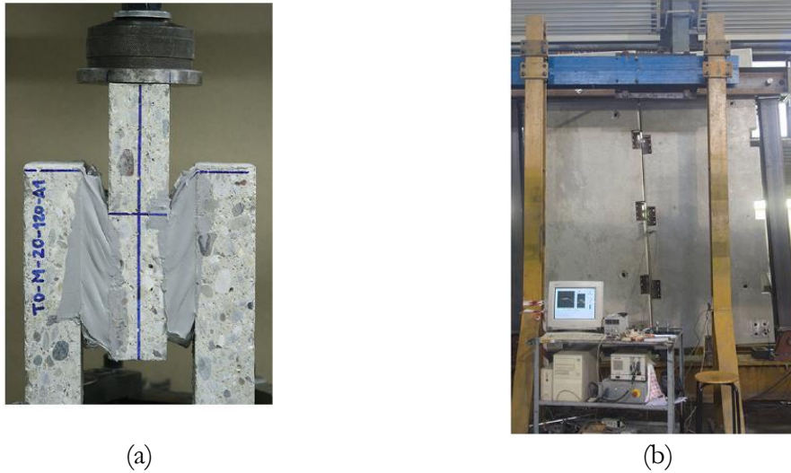
Figure 2-32: Local test on silicone (a) and pseudo-dynamic test on vertical panels sub-assembly
