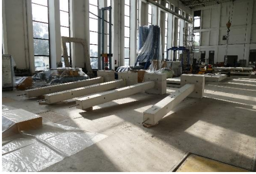
The four columns with \Phi 25 bar at the top for slab anchoring
