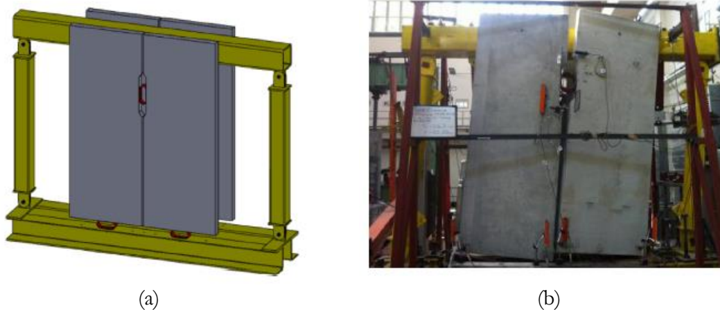
Figure 2-29: Steel Cushion connection test: sub-assembly test arrangement (a) and test picture (b). From (Karadoğan et al., 2019)
