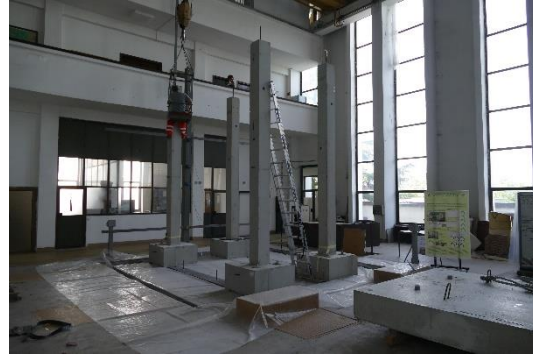
Columns installed on the shaking table
