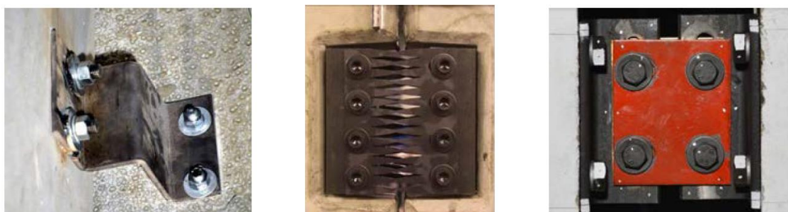
Figure 2-28: Folded Plate Device (a), Multiple Slit Device (b) and Friction Based Device from (Biondini et al., 2017)
