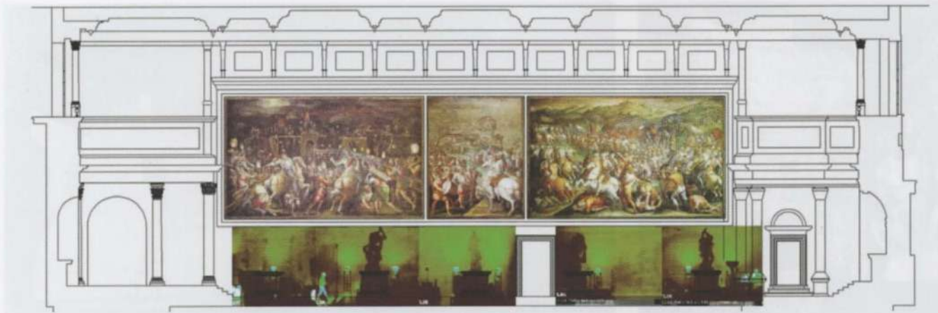
Figure 2. GIS project with thermal images showing masonry structure and the existing infilled openings.
