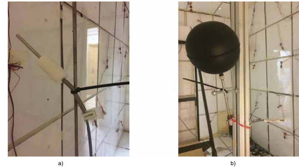
Fig.4. Pictures of: a) The globe thermometer to measure indoor radiant temperature; b) The PT100 thermoresistance to measure indoor air temperature
