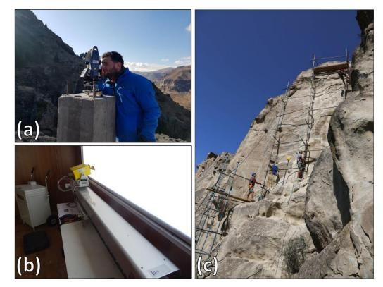
**Figure 19.** Nonstructural measures, such as displacement monitoring systems, planned in David Gareja: Robotized Total Station (**a**); ground based interferometric synthetic aperture radar system (**b**). The scaffolding constructed for the anchoring phase in Uplistsikhe (**c**).
