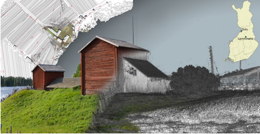
Fig. 5 The historic village of Lamminaho has represented a pilot project for the “Preserving Wooden Heritage” European Project. Starting from laser scanning survey activities it has been developed a detailed scientific report with the representation and description of all the buildings preserved in this area. A sort of technical dossier available for technicians and experts, responsible for the preservation of this Heritage
