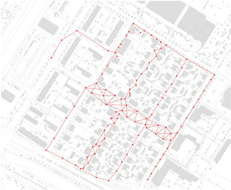
Fig. 13 Scan positions of the laser scanning survey of the wooden district of Raksila in Oulu, Finland. The main aim of the survey has been the study of the streets facades of this historic place and the recognition of the present townscape
