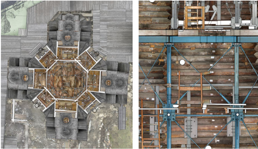
Fig. 17 Post production results of the case study of the Church of the Transfiguration. In order to understand the wooden structure nine floor plans and four sections were produced by elaborating orthophotos by using the photo documentation elaborated on field and detailed technical drawings
