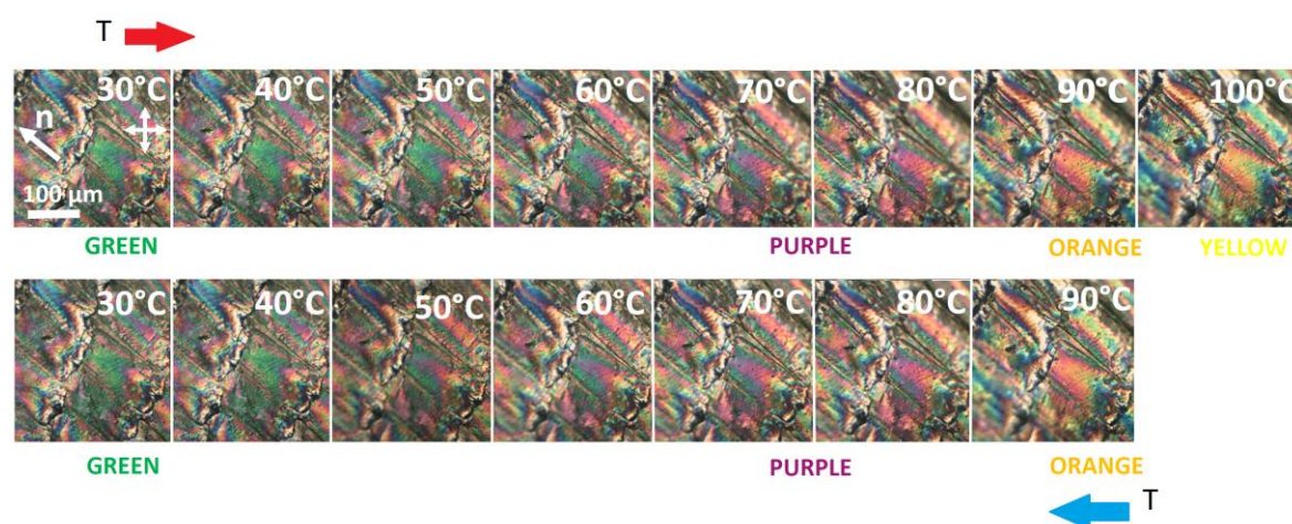
Figure 6.22. LCE scales are heated from room temperature until 100^\circ\text{C} showing color interference variations at POM. Decreasing the temperature until 30^\circ\text{C} , the sample recovers the same colors and therefore the initial birefringence.
