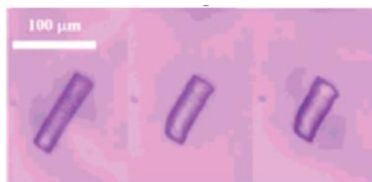
Figure 1.3. An isolated pillar exhibits a contraction with the order of 35%. Adapted from reference [13].
