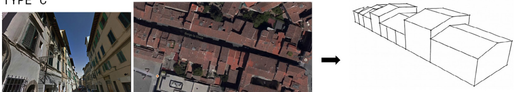
Figure 7 – Some examples of reconstructed buildings, divided in TYPE A: higher number of fonts and more precise informations, so more details and higher level of definiton of graphical representation; TYPE B: lower number of fonts and less precise informations, so less detail and lower level of definition of grapical representation; TYPE C: no fonts or not enough informations, so basic and simple representation.
