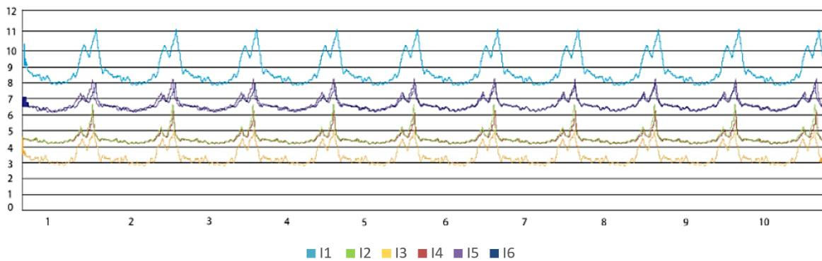
Figure 3. Water content kg/m<sup>3</sup> in the internal plaster layer on the wall M1-brick masonry for the climate of Florence
