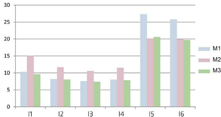
Figure 4. Comparison of total water content (kg/m<sup>3</sup>) inside the wall for M1- M2 - M3 envelope solutions for the climate of Florence
