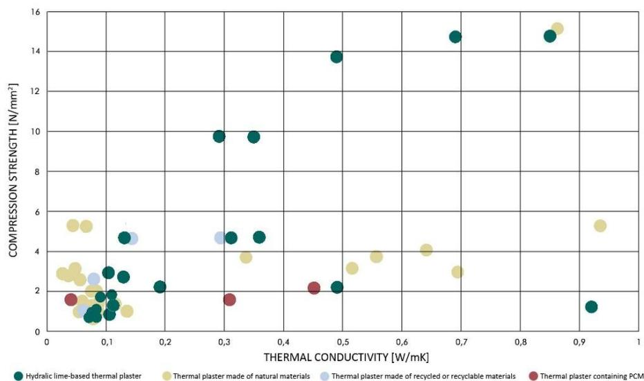
Figure 1. Thermal plasters investigated and compared considering the relation between the compression strength  $\sigma$  (N/mm<sup>2</sup>) and the thermal conductivity  $\lambda$  (W/mK) (Romano, Alecci et al, 2021)
