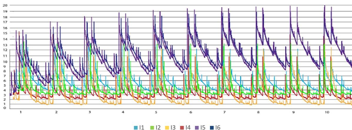
Figure 2. Total Water content (kg/m<sup>3</sup>) inside the wall M1-brick masonry for the climate of Florence
