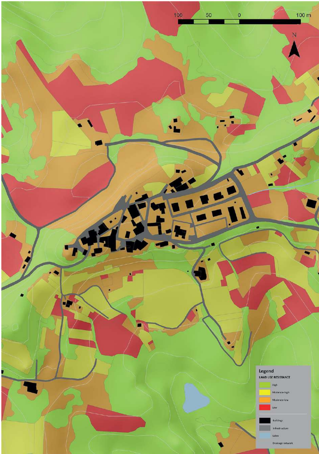
Ricasoli Map 13c – Land use resistance to earth slides and earth falls (Ricasoli village). In the figure, a detail of the original map is reported.
