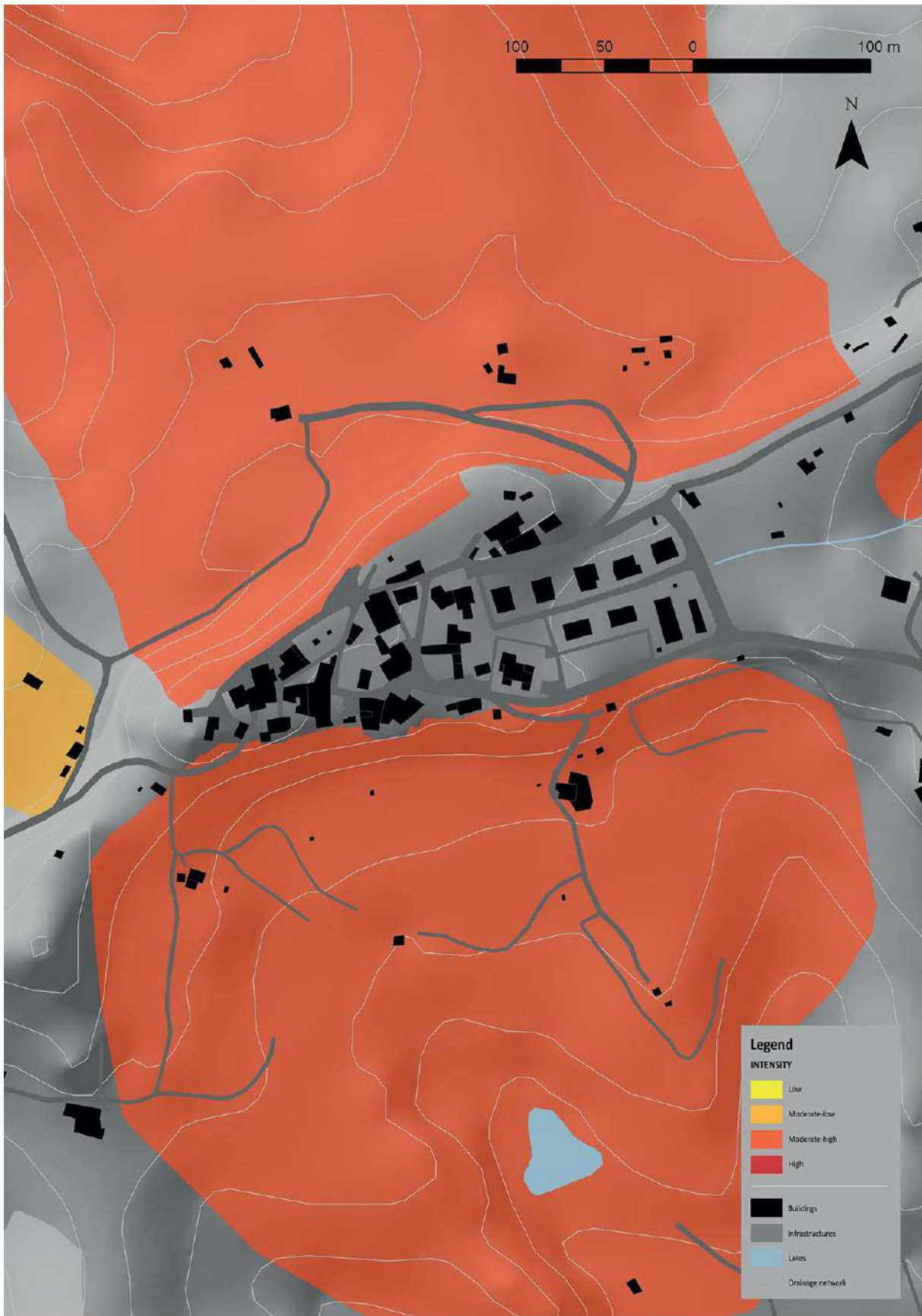
Ricasoli Map 10 – Earth slide intensity, expected scenario (Ricasoli village). In the figure, a detail of the original map is reported (modified after DST – UNIFI, 2009).
