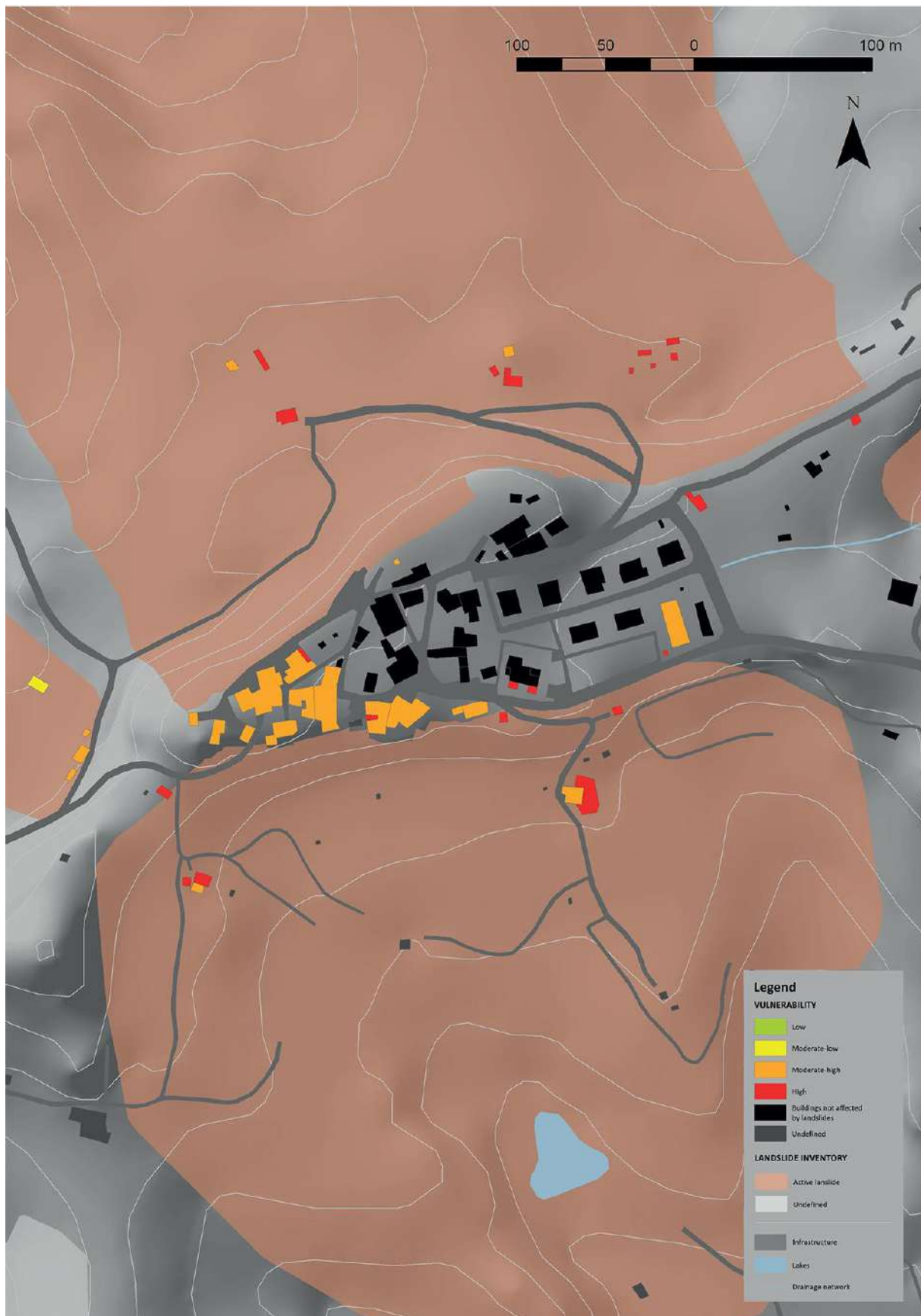
Ricasoli Map 14a – Physical vulnerability of buildings exposed to earth slides (expected scenario) (Ricasoli village).
