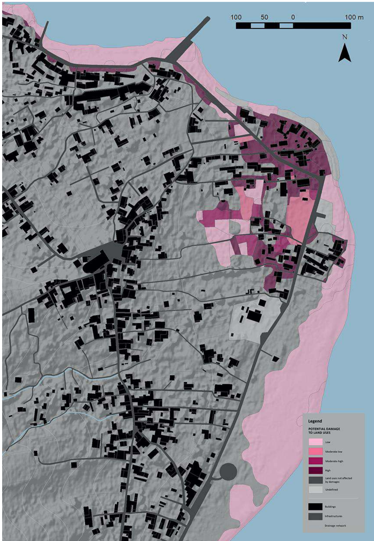
Stromboli Map 28b – Potential damage to land uses exposed to tsunamis (expected scenario: submarine landslide, 15 mln m 3 ) (Stromboli village).
