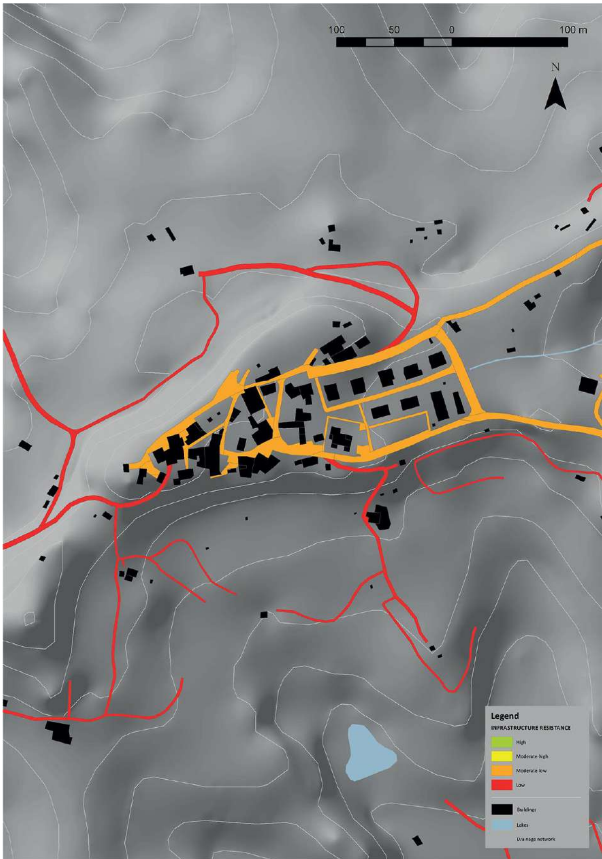
Ricasoli Map 13b – Infrastructure resistance to earth slides and earth falls (Ricasoli village). In the figure, a detail of the original map is reported.
