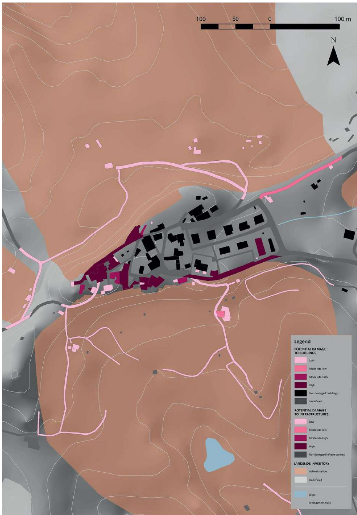
Ricasoli Map 20a – Potential damage to buildings and infrastructures exposed to earth slides (expected scenario) (Ricasoli village).
