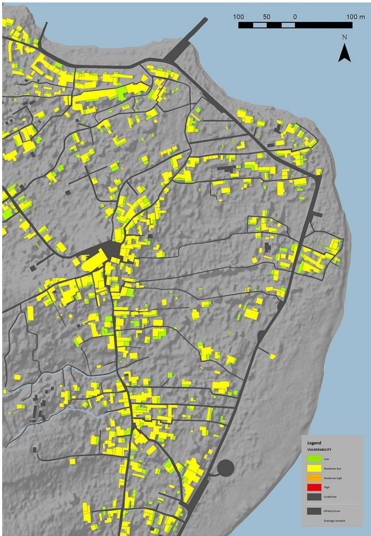
Stromboli Map 22a – Physical vulnerability of buildings exposed to earthquakes (expected scenario) (Stromboli village).
