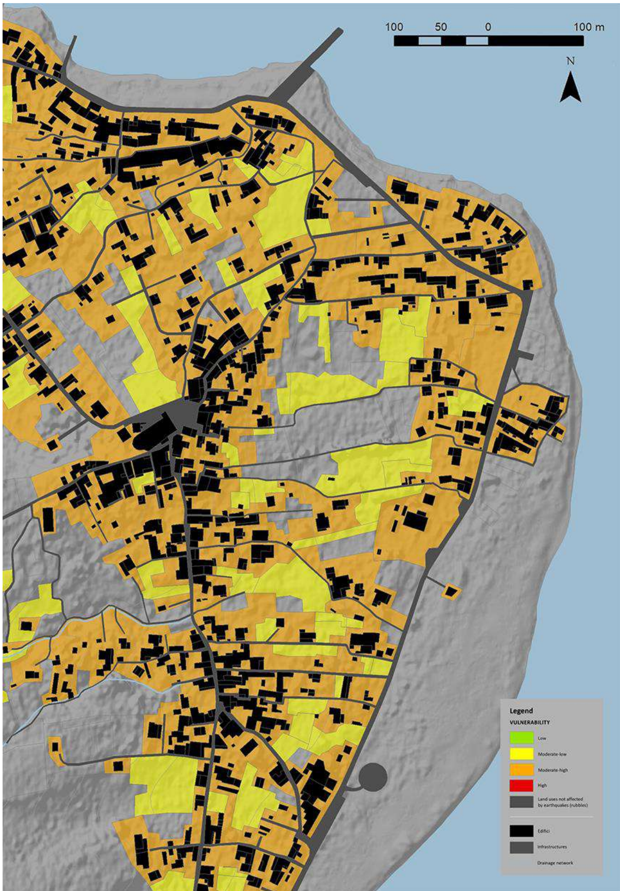
Stromboli Map 22c – Physical vulnerability of land uses exposed to earthquakes (expected scenario) (Stromboli village).
