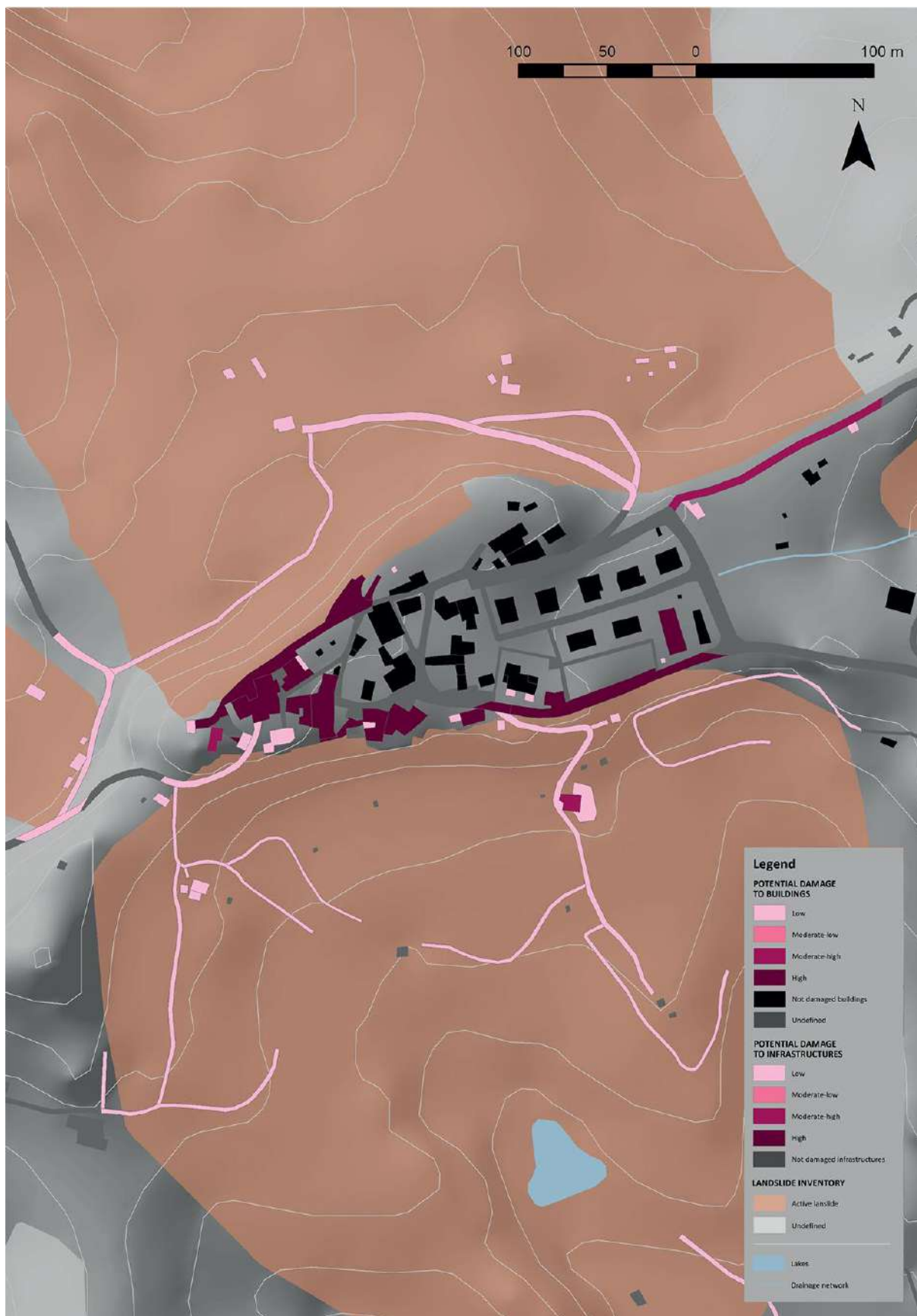
Ricasoli Map 21a – Potential damage to buildings and infrastructures exposed to earth slides (worst case scenario) (Ricasoli village).
