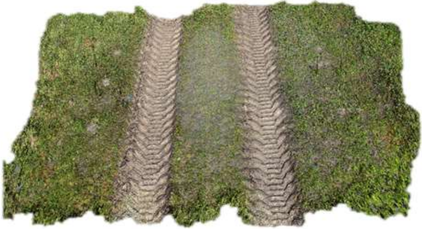
Figure 3.5. Image-based points cloud derived by SfM Photogrammetry by Agisoft PhotoScan software after 60 forwarder passages.
