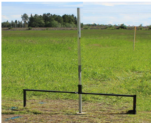
Figure 5.2. Manual instrument for rutting measurements.
