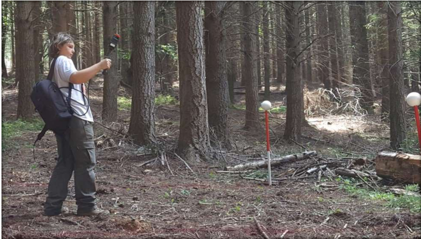
Figure 4.4. Operator during laser scanner survey, holding and oscillating the instrument at breast height (1.30 m above ground) while walking.
