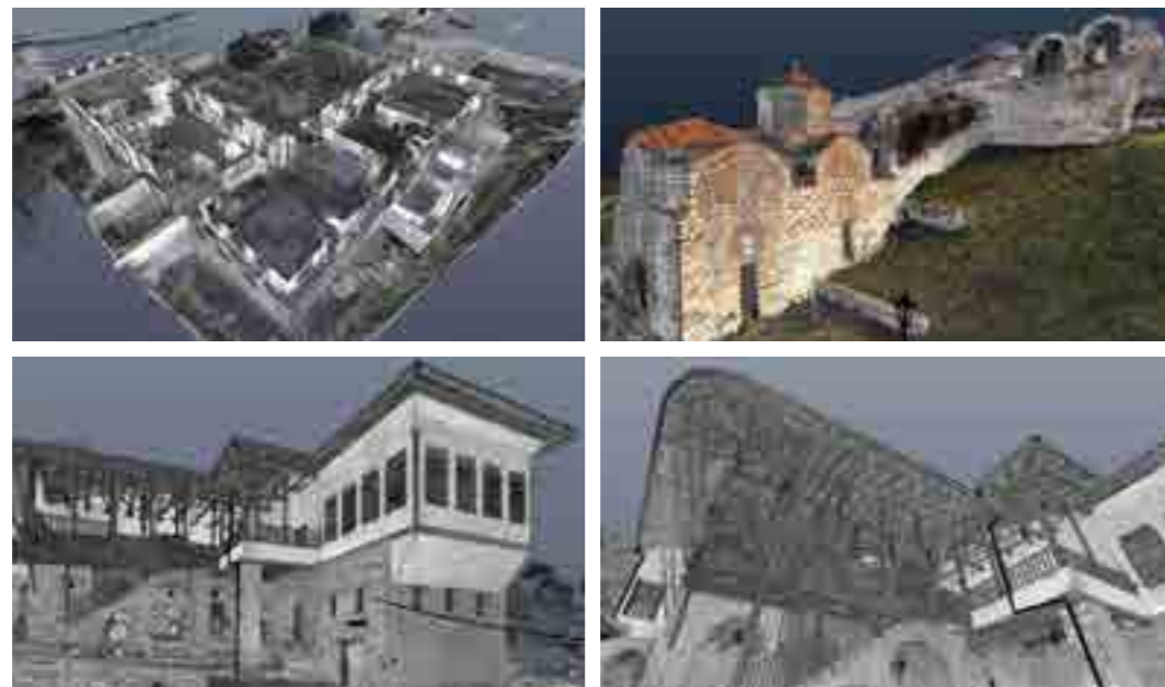
Berat, 3D Laser Scanner digital survey of Berat, lasergrammetry of the Holy Trinity Church and the Ethnographic Museum (© G. Verdiani, F. Tioli, UNIZKM, DIDA, 2020)
