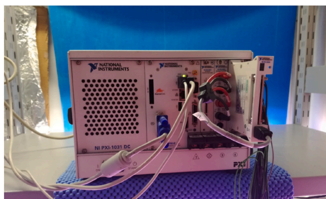
Fig. 2. National Instruments data acquisition card connected to the electrodes for measuring plant electrical activity.
