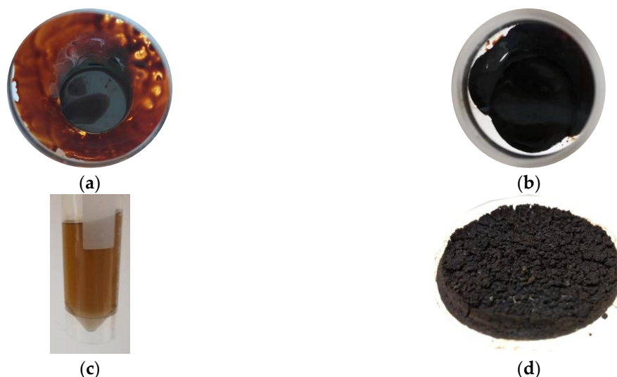
Figure 34. Products collected from a typical hydrothermal liquefaction (HTL) experiment in the micro-batch reactors: light biocrude or BC1 (a), heavy biocrude or BC2 (b), aqueous phase with water-soluble organics (WSO) (c) and solid residue (d).
