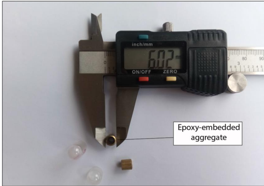
Fig. 2.7 Conductive brass tubes used for the micro-CT analysis of aggregates.
