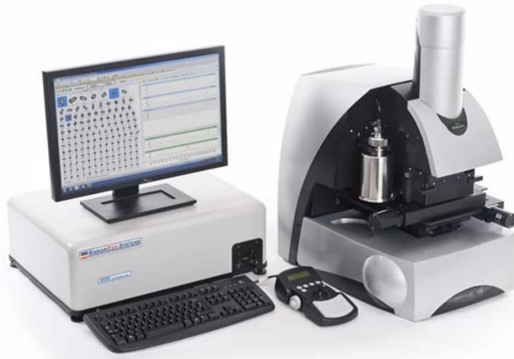
Fig. 2.1 Morphologi G3se, from Malvern Panalytical™.
