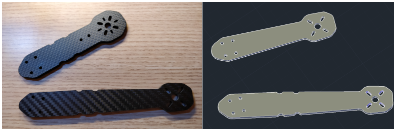
Figure 3.11: In the image it is possible to observe the two versions of arms, where the custom arm is the longer one. The finished carbon fiber arms are shown on the left side of the figure (standard version and customized version). On the right side of the figure there is a CAD view of the two versions of the arm. For the realization of the customized arm, a carbon fiber plate suitably worked by means of a CNC milling machine was used.
