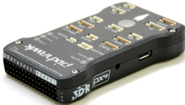
Figure 2.1: The figure shows the PixHawk open-source autopilot board. This microcontroller is suitably customized for use on drones, in normal use it is able to automatically stabilize the attitude and control the altitude. If required, it can carry out simple automatic missions based on the use of GPS technology.
