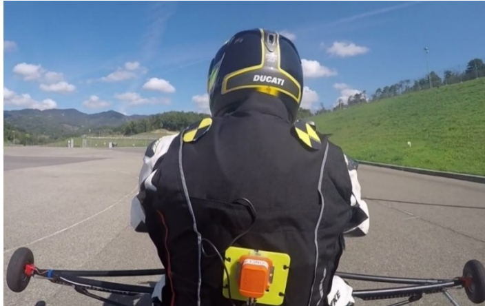
Figure 25 – Xsens MTi-G IMU position (orange in the back) and markers on the back of the rider
