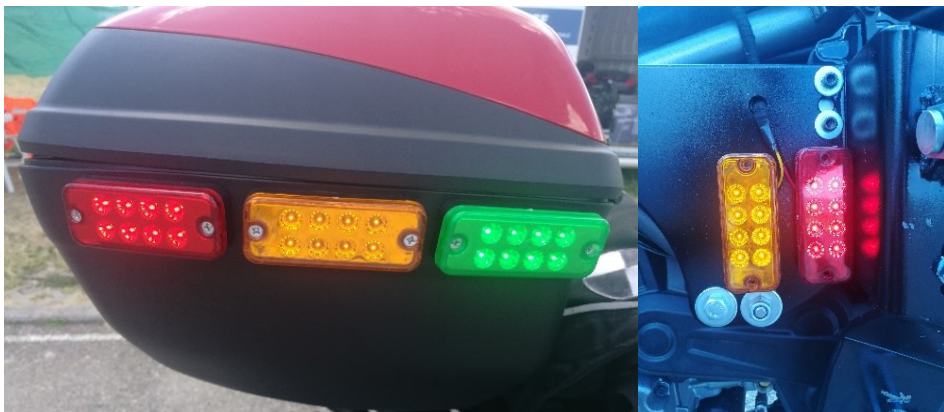
Figure 24 – Information lights: Level of AB intervention (SX), Status of the AB system (DX)
