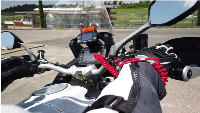
Figure 23 – Kill-Switch with elastic cord secured around the rider's wrist
