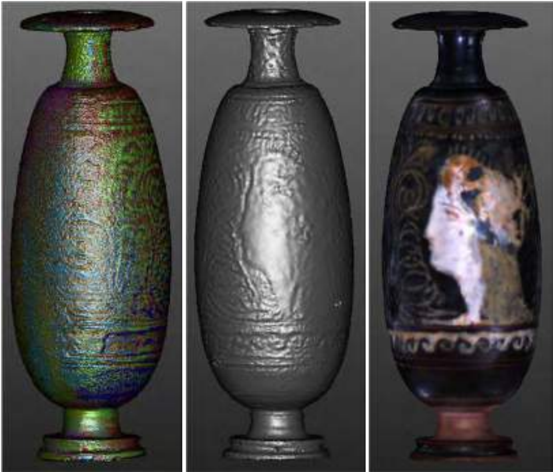
Fig. 2: the data collected by the scanner are X, Y, Z coordinate triplets of each single point acquired, taking a set of partially overlapping range scans. Different colours represent the contribution of each different scan (on the left). The points were triangulated in order to obtain the polygon mesh, a collection of vertices, edges and faces that defines the shape of the artefact (in the middle). The result is a 3D very high resolution and photorealistic model (on the right).
