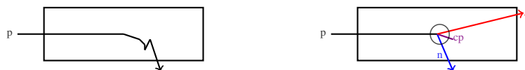
Fig. 4.7 (a) (Multiple-) Elastic scattering effect. (b) Reaction and/or inelastic scattering effects. Here p stands for proton, cp for charged particles and n/\gamma for neutrons and gamma-rays.
