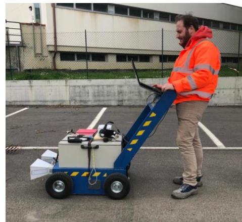
Fig. 15. ORFEUS modified with the additional antennas.
