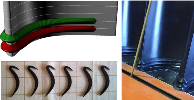
Figure 5.10: CAD representation of the fences, manufactured fences via rapid prototyping and the linear cascade with fenced blades
