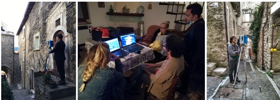
Figure 1 - The 3D laser scanner unit at work and first in place data treatment with importing and alignment in Autodesk Recap (© S. Giraudeau, G. Verdiani, A. Leonardi).
