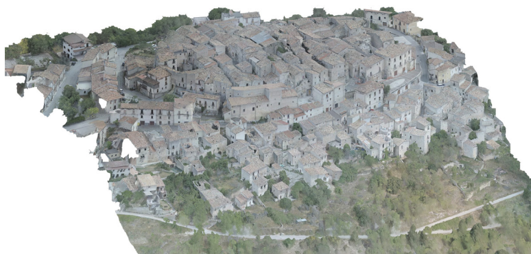
Figure 11. Aerial survey result, developed with Agisoft Metashape; 35.389.799 Faces; 17.727.890 Vertices (© S. Giraudeau, A. Leonardi, G. Verdiani).
