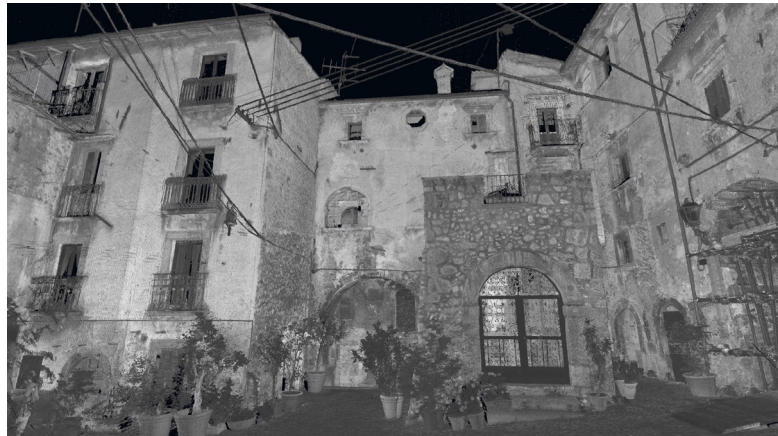
Figure 2 - View of the aligned point clouds in Autodesk Recap (© S. Giraudeau, G. Verdiani, A. Leonardi).
