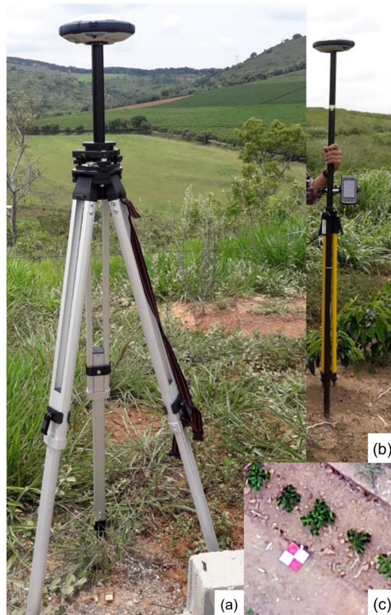
Figure 4. Equipment used for control points georeferencing. (a) GNSS receiver (base), (b) GNSS receiver (Rover) RTK mode, (c): ground control points (GCPs).
