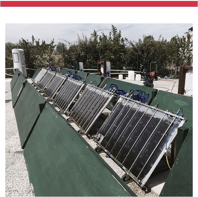
Figure 1. GWP®-III reactors installed at the experimental area of Fotosintetica & Microbiologica S.r.l. (Sesto Fiorentino, Florence, Italy). Dummies are placed in front, back, and sides of the reactors to simulate a full-scale plant. The panels face south with an inclination of 50°. The distance between rows is 1 m.
