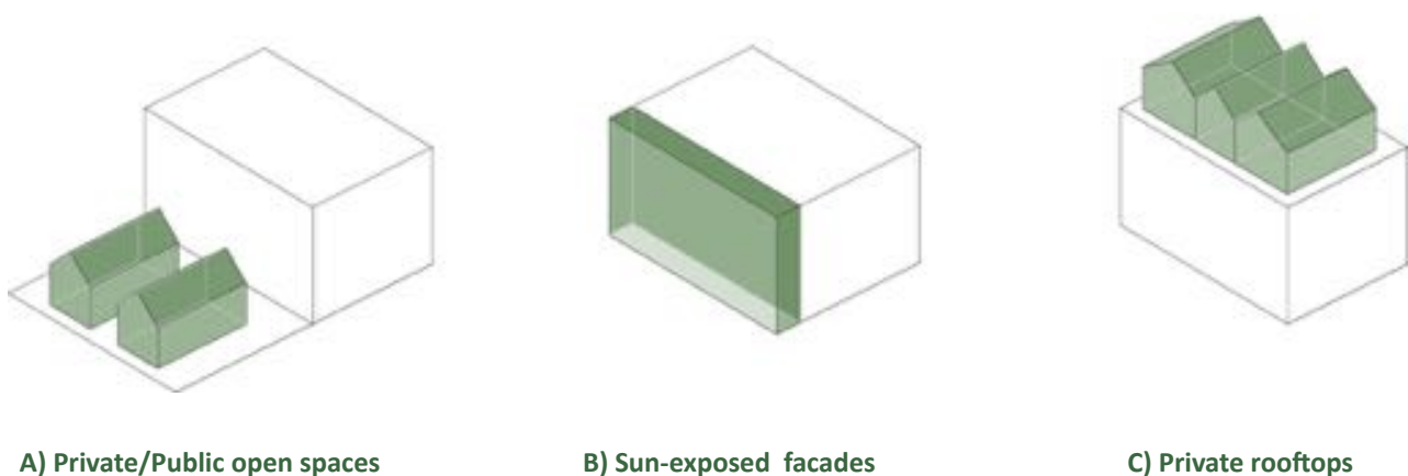
Fig. 8: High-tech Greenhouse integration in buildings
