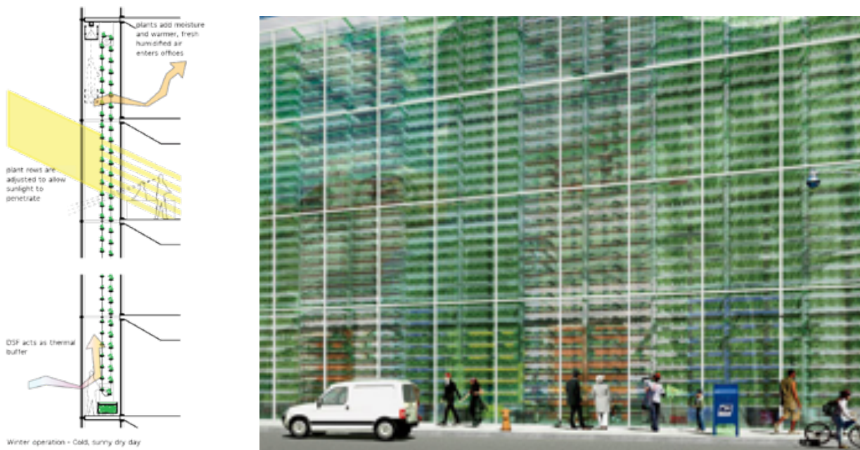
Fig. 10: Experimentations for a productive facades. Building integrated hydroponic food market - Abu Dhabi. Kiss+Cathcart Architects
