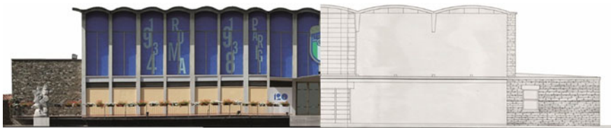
Fig. 7 Comparison of the original project graphs and the representation of the current state of fact of the gym of the Federal Technical Center of Coverciano
