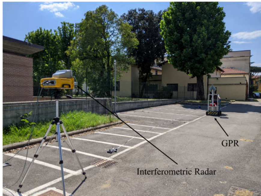
Figure 8. Experimental setup for GPR positioning by interferometric radar.
