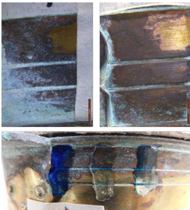
Figure 50. Diocesan bucket before (top left) and after (top right) the cleaning procedure. The bottom figure shows the application of the HVPDs loaded with TEPA 3% and EDTA 0.1 M. It must be notice that the viscosity of the systems allows the application also on vertical surfaces.
