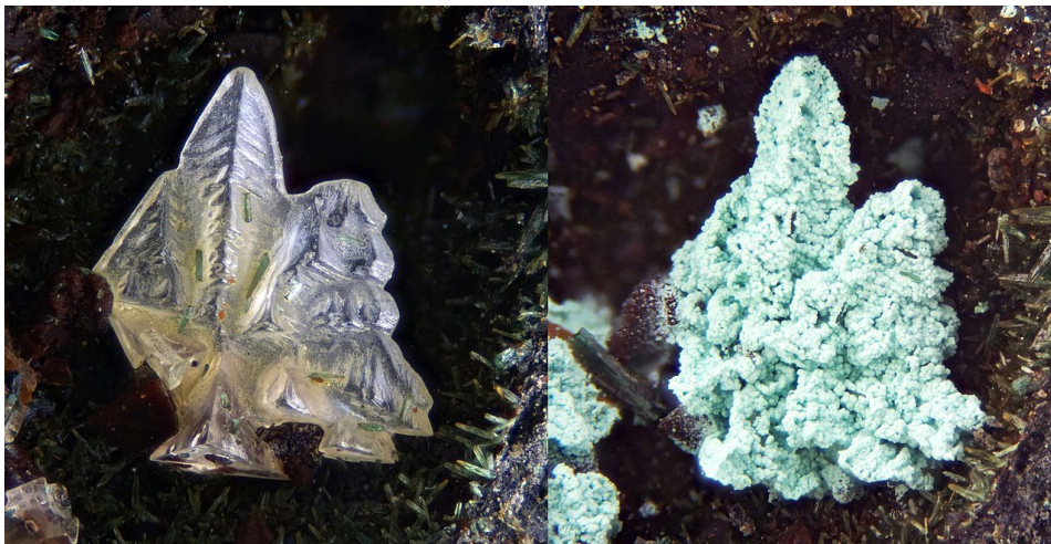
Figure 15. Conversion of nantokite (left) to atacamite (right) after reaction with oxygen and moisture.
