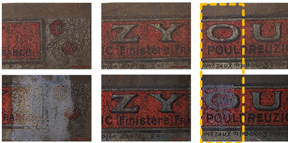
Figure 53. Decorated tin box before (top) and after (bottom) the cleaning procedure. Area treated with the HVPD (left) and pHEMA/PVP semi-IPN (centre) both loaded with citric acid solution (1% w/w). Area treated with pHEMA/PVP semi-IPN loaded with TEPA (3% w/w) (yellow).
