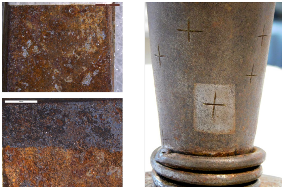
Figure 51. Iron chalice before (top left) and after (bottom left) the treatment with HVPD loaded with citric acid (10% w/w). Figure on the right shows the results obtained after the application of pHEMA/PVP semi-IPN loaded with the citric acid (10% w/w) solution.
