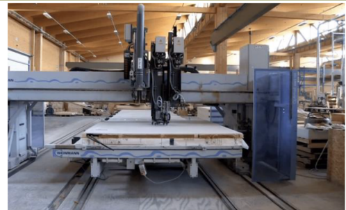
Image 01 – Panels are assembled by pressing and adhesive following streamline sequences of industrial operations
