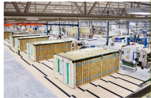
Image 02 – Modular units are off-site manufactured following streamline sequences of assembly
