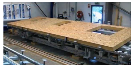
Image 02 – Panels are assembled inside a factory, where they are provided with holes for allocating services, windows and doors. This limit possibility for future integration and modifications
