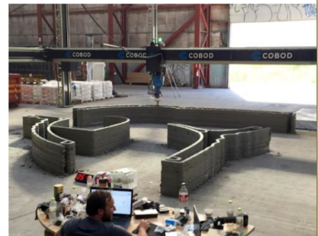
Image 02 – Automated printing process: human interaction is limited to machine setting and control Credits: COBOD
