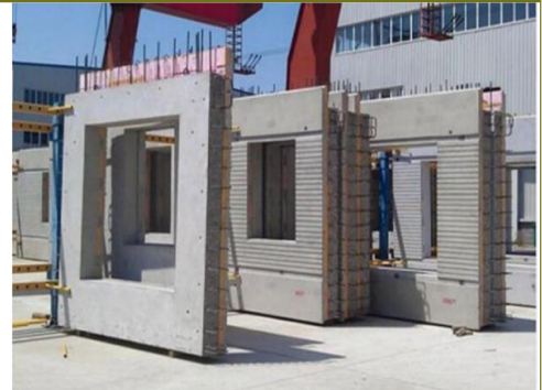
Image 01 – Precast concrete panels can be off-site manufactured and finished with different degrees of prefabrication (from raw structural panels to those integrated with doors and windows)
