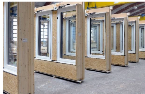
Image 02 – CLT panels are off-site manufactured in batches and then shipped for installation on site
