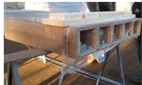
Image 02 – Cardboard panels are infilled with eco-friendly and recycled insulation Credits: E. Belardi
