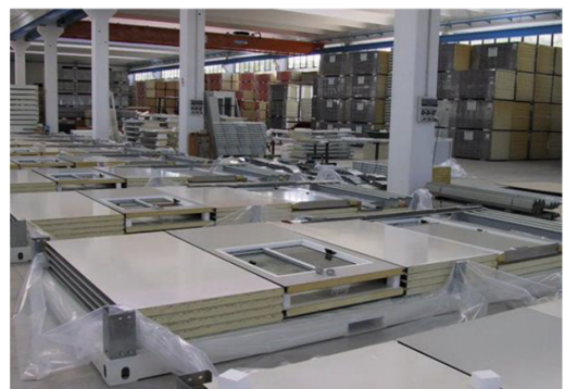
Image 03 – Portable units in “flat-packed” delivering option are mass-produced in batches and stocked for orders
