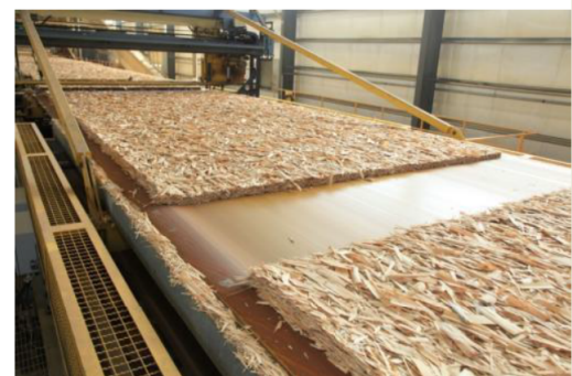
Image 03 – OSB panels used to encase insulation are produced gluing together wooden shreds coming from production wastes, offering the opportunity to reduce the use of raw materials
