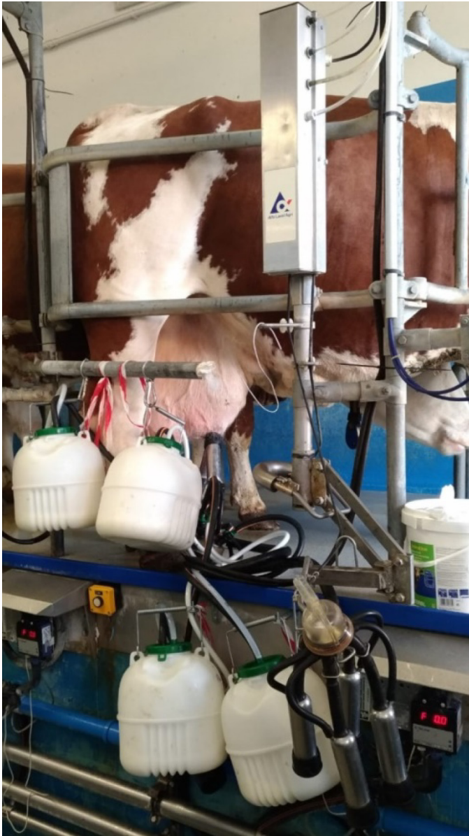
Figure 1. Vacuum system connected to 4 different buckets used in the study to simultaneously drain the 4 quarters.
