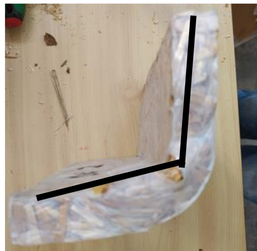
Figure 11. Bending results with preheating conditions and central groove.
