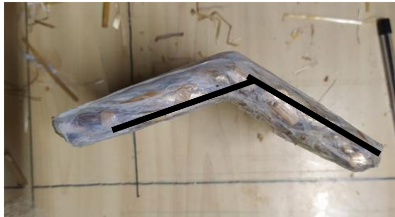
Figure 9. Bending results with pre-heating conditions.
