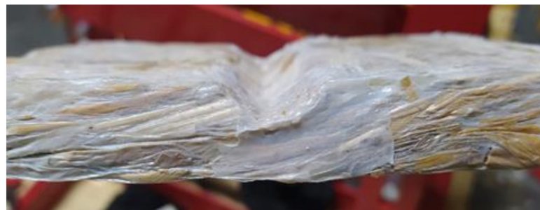
Figure 10. Central groove created to ease the bending process.
