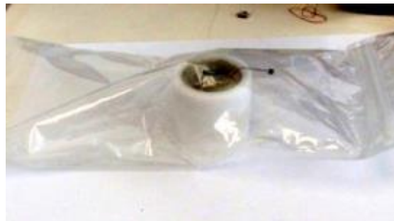
Fig. 6. Transparent envelop with inside the dedicated irradiation LED support and the H. pylori cultures (idle).
