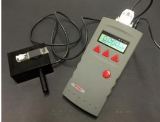
Fig. 3. Experimental setup for the measurement of the radiant flux. Left: integrating sphere where the LED is placed for testing. Right: power meter.
