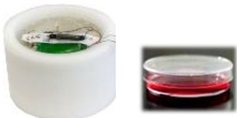
Fig. 5. Dedicated LED support for in vitro irradiation (left) of H.pylori cultures (right).
