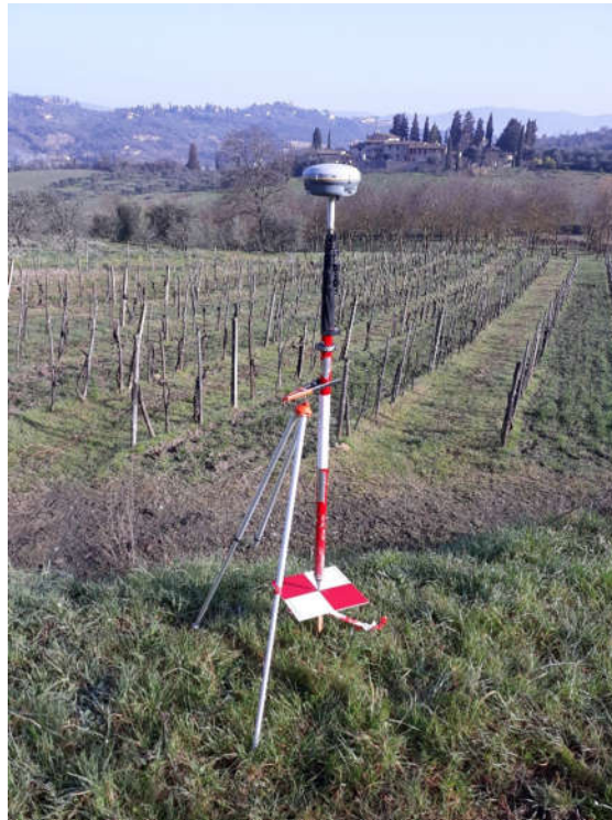
Figure 2. Measuring session of a ground target with pole, GNSS antenna and bipod.
