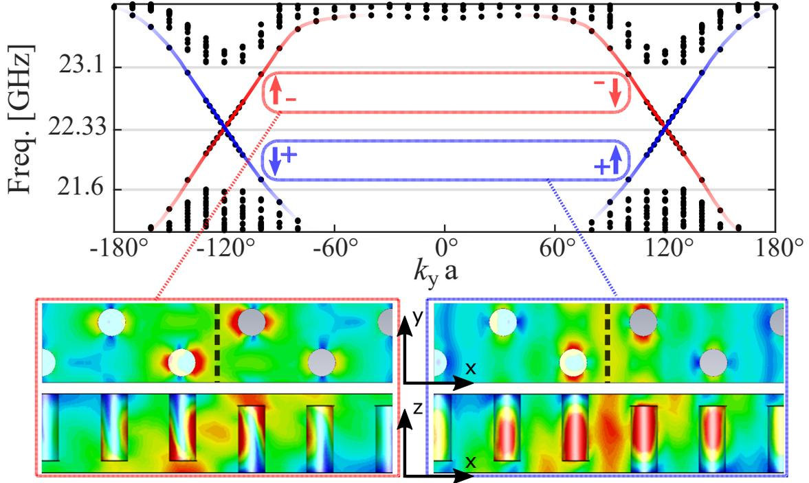
Fig. 2. (color online) **Top:** PBS of the topological interface. Arrows are spin states and signs are modal effective index sign. **Bottom:** Electric field amplitude in the longitudinal and transverse direction for the TPHEMs. The spin state is determined by the time evolution of the electric field in the air gap region.
