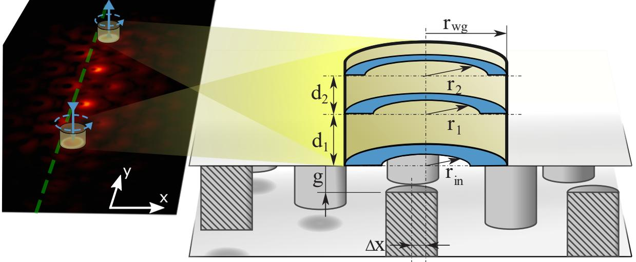
Fig. 3. (color online) **left:** Absolute value of the Poynting vector for a TPHEM propagating from a CWG launcher to a second one placed at a distance of  $9a_0$ . **right:** Schematic of the CWG launcher.
