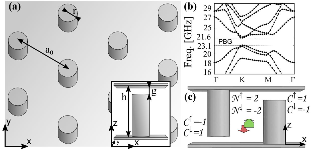
Fig. 1. (a) Schematic of TPhC,  $a_0 = 10\text{mm}$ ,  $r = 1.725a_0$ ,  $g = 0.15a_0$ ,  $h = a_0$ . (b) Photonic Band Structure (PBS) of the TPhC with the complete PBG highlighted. (c) Topological interface between two  $z$ -symmetry reversed TPhCs. The number of unidirectional edge modes for every spin state is given by the difference between the confining spin-Chern Numbers.
