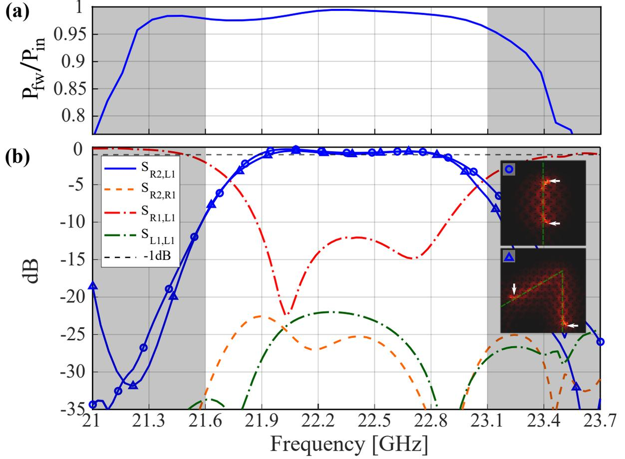
Fig. 4. (color online) (a) Ratio between Fw and total outgoing power as a function of excitation frequency. (b) *Solid lines*: LCP-to-RCP transmission of the straight (circles) and bent (triangles) TPMWs. *Dash-point*: Single port co and cross polarization reflection coefficients. *Short dash*: RCP-to-RCP transmission of the straight TPMW. *Inset*: Poynting vector at  $z = h/2$ ; TPMW is indicated with green short-dash line while white arrows indicate CWG launchers positions.
