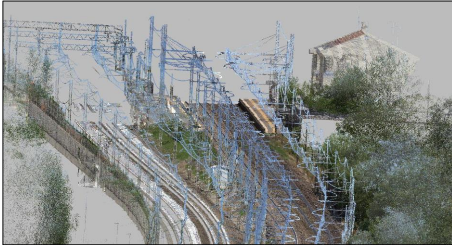
Figure 52 – “Example of train mobile mapping point cloud acquired in the proximity of a station” (Corongiu et al., 2020)
