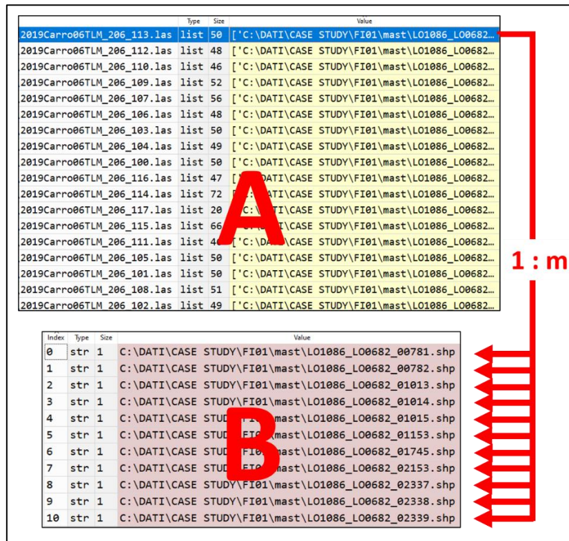
Figure 47 - Dictionary set up: table A represent the list of LAS files, table B represent the list of SHP assets connected with each row of table A. Between table A and table B a one-to-many (1:m) relationship there exists
