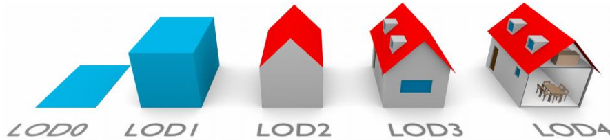
Figure 5 - Building CityGML LODs (Biljecki et al., 2016)
