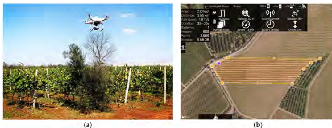
Figure 6. UAV aerial data acquisition: (a) DJI Phantom 3 Professional UAV in the vineyard; (b) UAV photogrammetry mission over the vineyard (Map Pilot app) with the overview of the interface for the flight mission and parameters. The yellow lines indicate the borders of the survey area, the green and red placemarks indicate the mission start and end points, respectively, and the purple placemark indicate the UAV take-off/landing point (i.e., the UAV pilot position).
