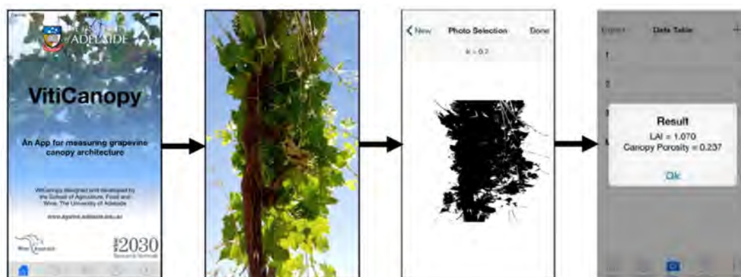
Figure 3. Example of Leaf Area Index (LAI) measurement procedure using the VitiCanopy app. From left to right, the app user interface, the shot image of the vine canopy, the segmented binary image of the canopy and the results in terms of LAI and canopy porosity.
