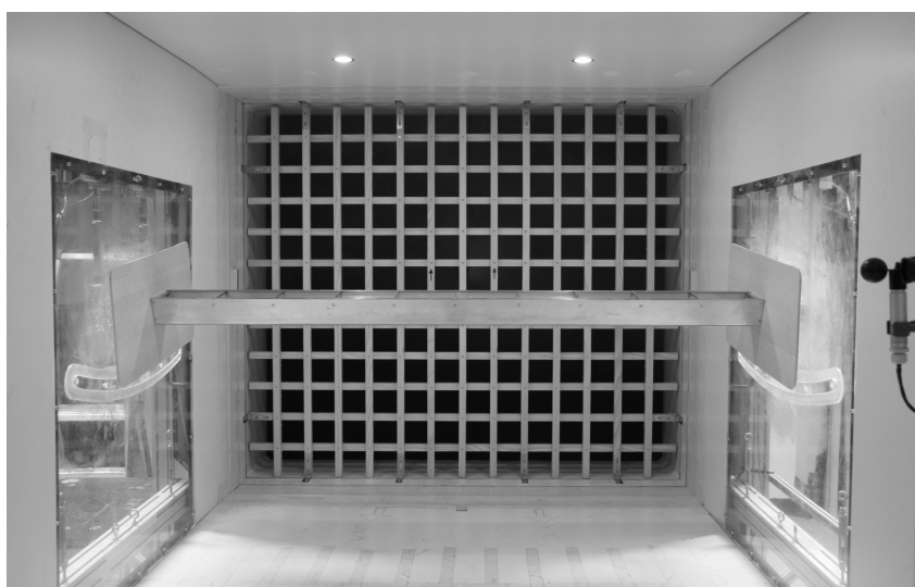
Fig. 3.11: Photo of the used turbulence grid (upstream of the wind tunnel model).
