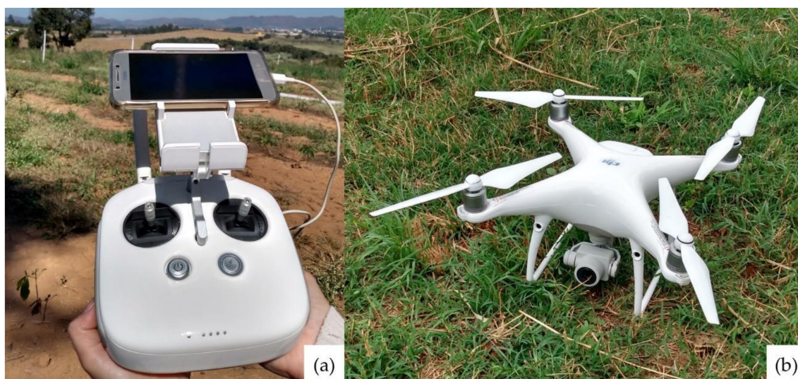
Figure 3. Equipment used to collect images, (a) radio control and (b) remotely piloted aircraft (RPA).
