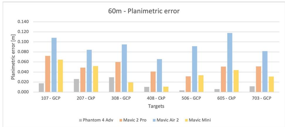
**Fig. 11** Chart of residuals on GCPs and CKPs of the four UAS
