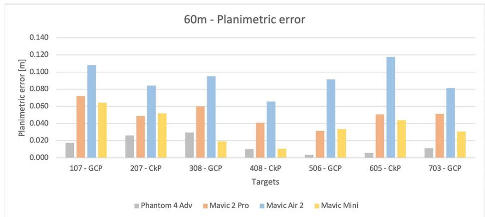
**Fig. 12** Chart of median calculated for planimetric error
