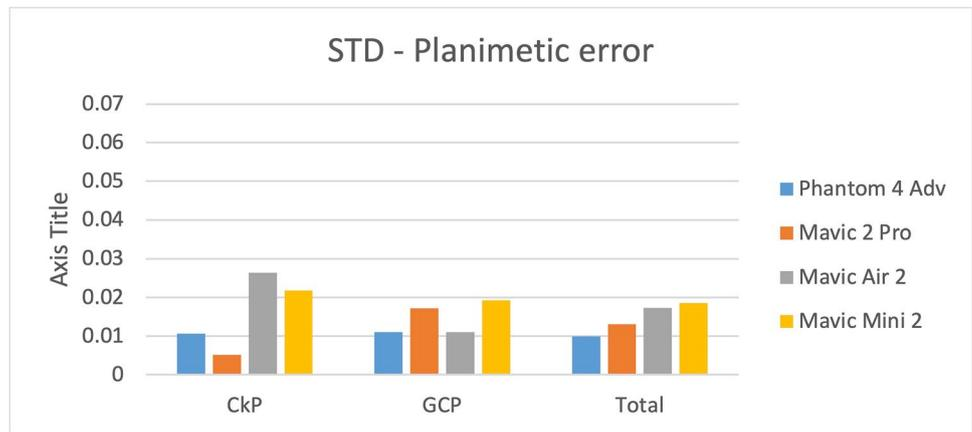
**Fig. 14** Chart of standard deviation calculated for planimetric errors
